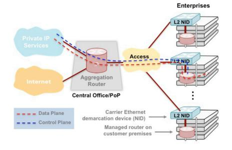
FIGURE 5 Traditional Managed Router Service requires expensive and difficult-to-manage customerlocated routers and an expensive central office router port for each customer endpoint.
