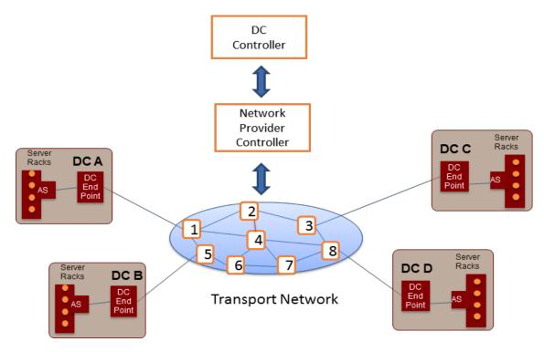
Figure 6 – Data center interconnection architecture
