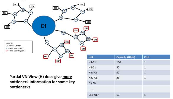
Figure A.4 – Partial graph topology view, high granularity
