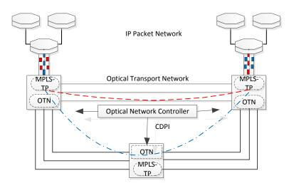
Figure 9 – Optical network with converged packet functions
