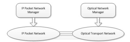
Figure 8 – Independent operation of packet and optical networks
