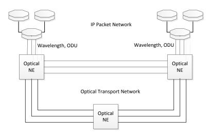
Figure 7 – Example of packet and optical networks
