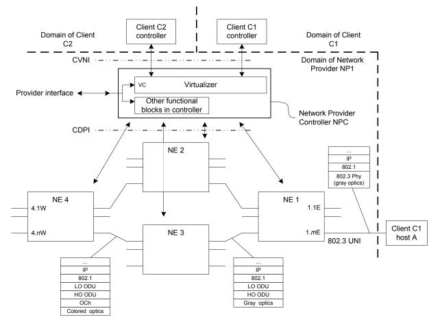
Figure 2 – Physical network, single provider domain
