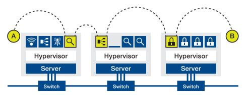
Today's hardware-based approach makes it extremely complex and time-consuming to implement service chaining, and expensive to scale and manage. Appliances must be physically installed and cabled, then assigned to physical domain qualifiers such as VLANs, sub-networks, etc., which typically limit their connectivity. Configuration must be manual and meticulous to implement the service chain.
