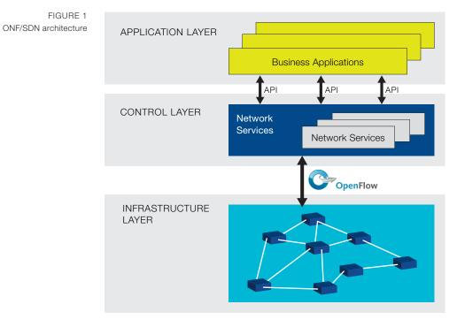
The ONF/SDN architecture consists of three distinct layers that are accessible through open APIs:
