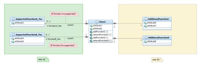
Figure 7.4: Flexible Attribute Assignment to Object Classes
