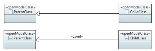
Figure 5.15: Generalization Relationship Notation (normal and conditional)
