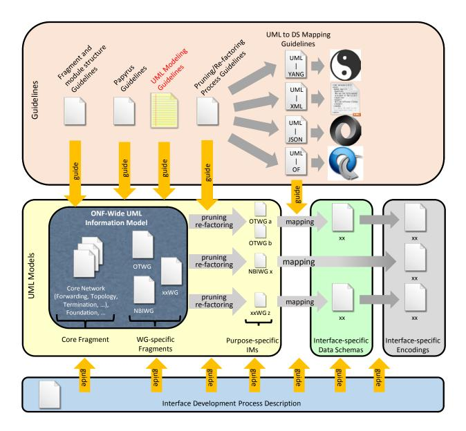
Figure 4.1: ONF Specification Architecture
