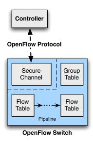
Figure 1: Main components of an OpenFlow switch.
