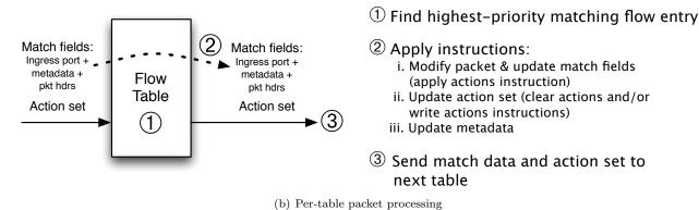
Figure 2: Packet flow through the processing pipeline
