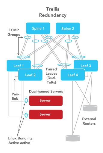
**Horizontal Scaling & Redundancy.** Trellis allows horizontal scaling of the fabric. Operators can start off with simply a single switch or two (for redundancy). As needs grow, they can add more spines and more leaves to their infrastructure seamlessly. This feature supports both scale and redundancy built into both spine and leaf layers as well as the control-plane which is based on a high-performance, scalable and resilient ONOS cluster.
