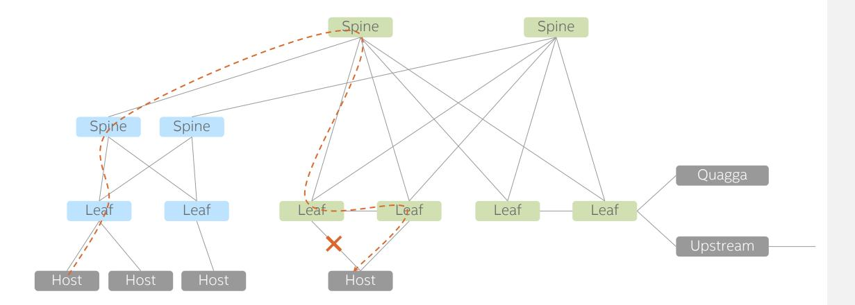
Pair link is only used to recover local failure
