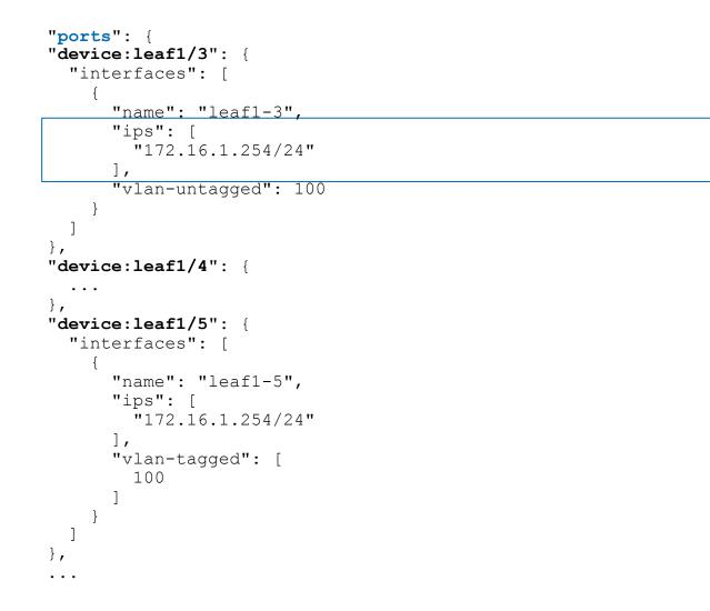
Two information can be derived from the subnet config:(1) The interface IP on the switch is 172.16.1.254(2) The subnet on this interface is 172.16.1.0/24
